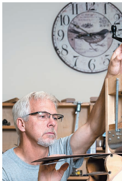
Beckwith prepares the sides of a guitar body in a special press.
